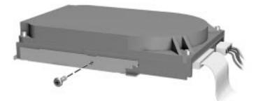
Slide the bracket into the molded plastic drive slot. Secure the bracket to the front panel with the two screws shown in "Removing the Bracket Screws."
